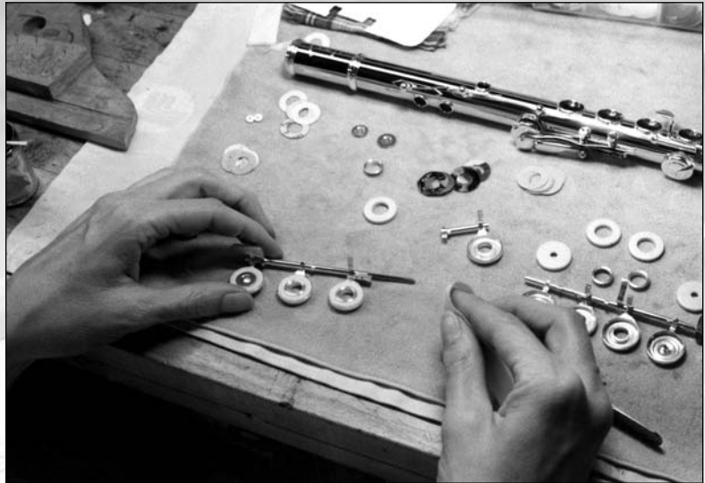
The jewels in your flute: paper shims, pad washers, and paper washers, among other parts.
